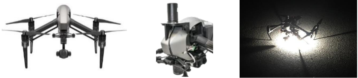
Figure 2. (Left) DJI Inspire 2 with X4S; (Middle) AirGon Loki Direct Geopositioning System; (Right) Inspire 2 at night
